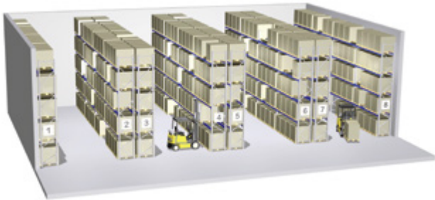
Pallet racks in a conventional arrangement
